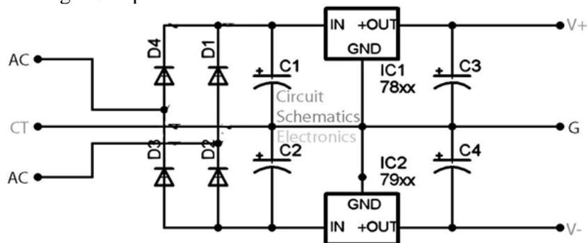
Figure 28.2 Dual Voltage Regulator
