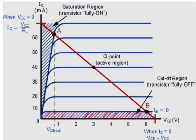
Figure15.1 : Operating regions of Transistor.
