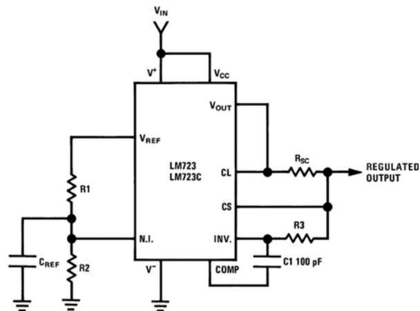
**Figure 29.3: Circuit diagram of IC LM723**
