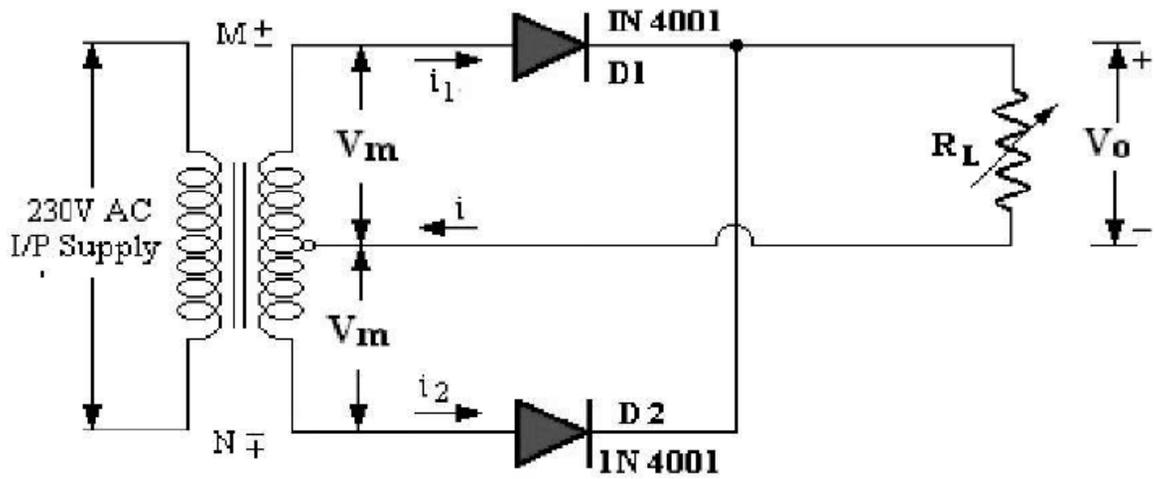
**Figure 6.1 : full wave rectifier with two diodes.**
