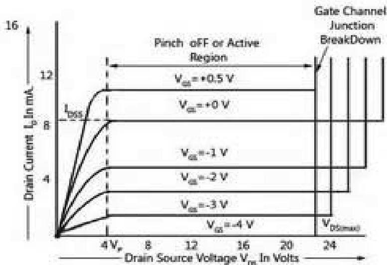
Figure 1: Drain characteristic
