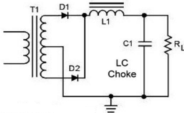
**Figure 8.1: Full wave rectifier with LC filter.**
