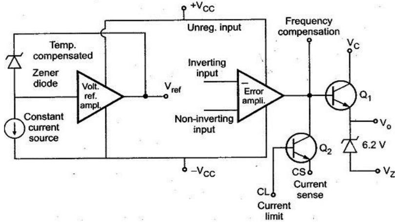
Figure 30.2: Block diagram of IC LM723
