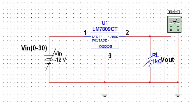
d. Actual circuit diagram used in Laboratory with equipment specifications.
