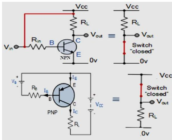
Figure 15.3 : Saturation region of Transistor.
