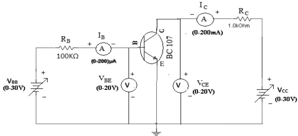
Figure 13.3: Circuit diagram of BJT in CE mode
