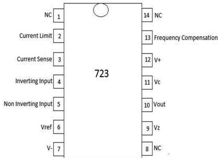
**Figure 30.1: Pin configuration of IC LM723**
