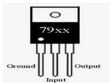
Figure 1 : negative voltage 79XX series IC
