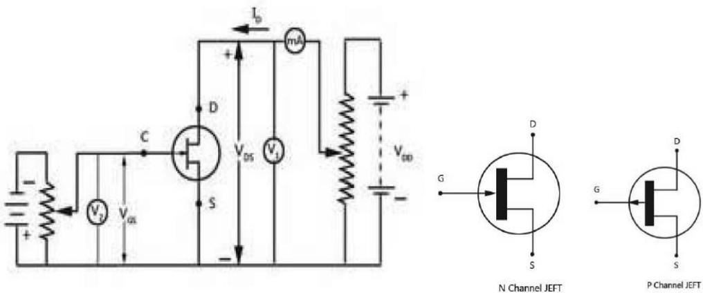
Figure 2: FET characteristic and its symbol
