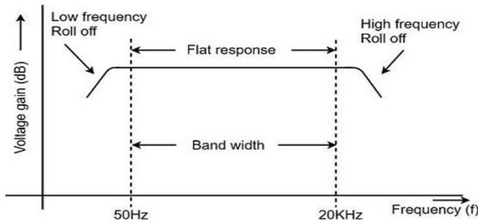
**FIGURE 18.1 FREQUENCY RESPONSE OF AMPLIFIER**
