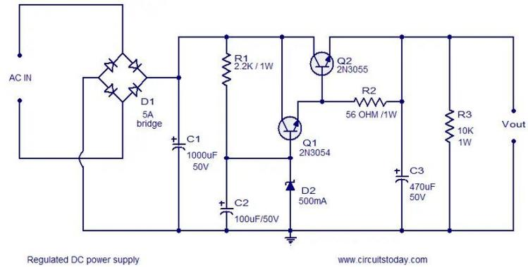
**Figure24.1: Regulated power supply**
