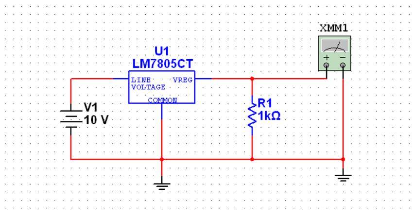
Figure 2 voltage regulator using 7805
