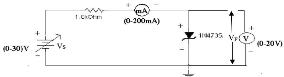
Figure 2: Circuit diagram of diode in forward bias
