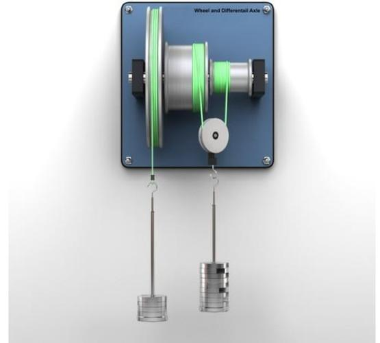
**Fig: Differential Axle and Wheel**
