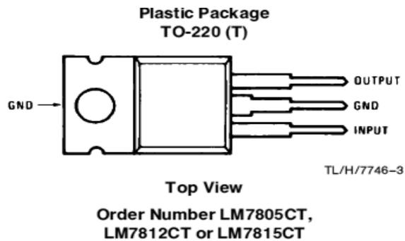
Figure 24.1: Pin diagram of IC78XX
