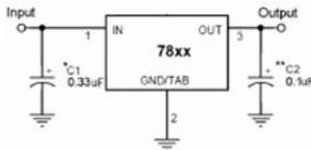
A common ground is required between the input and the output voltages. The input voltage must remain typically 2.0V above the output voltage even during the low point on the Input ripple voltage.
