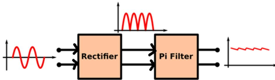
Figure 7.1: Concept of filter
