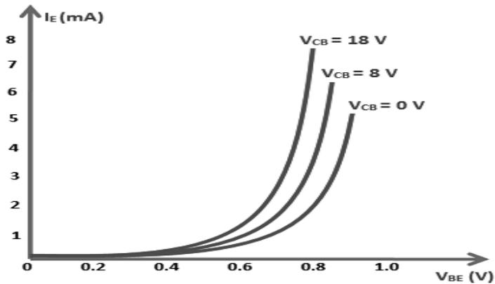
Figure 15.1: Input characteristics in CB
