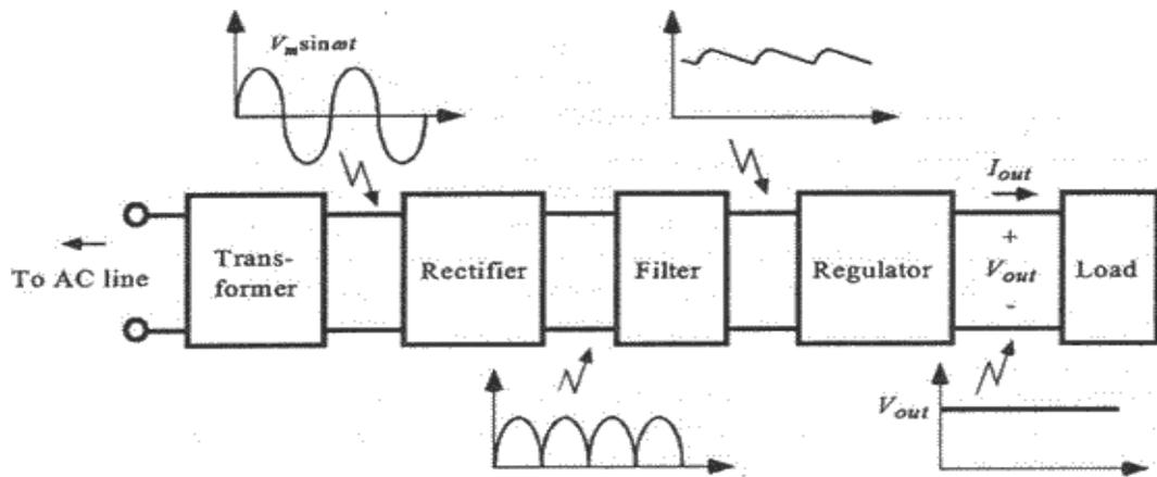
Figure 21.1: Block diagram of Regulated power supply
