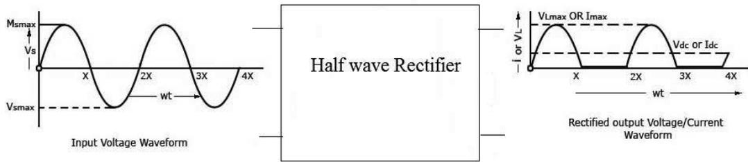
**Figure 6.2: Half wave Rectifier**
