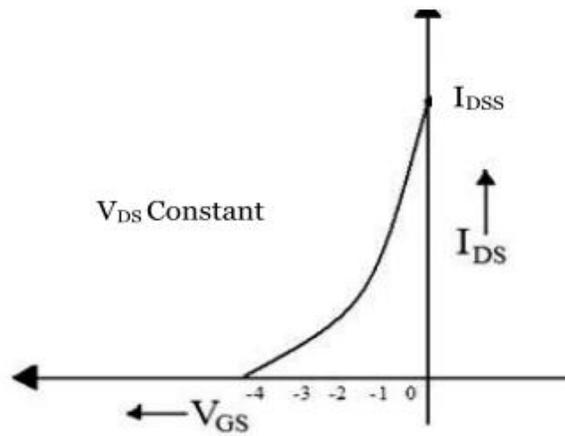
Figure 19.1: Transfer characteristics
