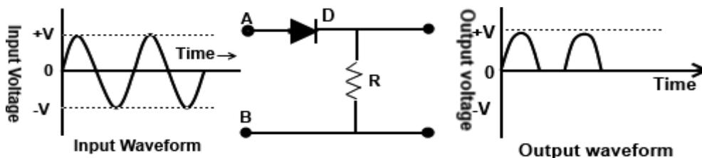
Figure 12.2: Circuit diagram of Negative Clipper.
