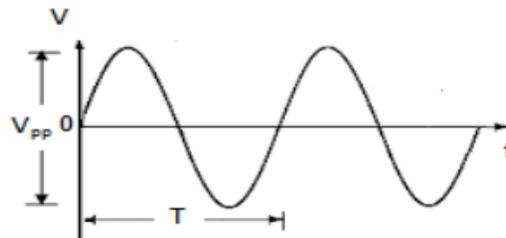
Figure 20.1: Sinusoidal output
