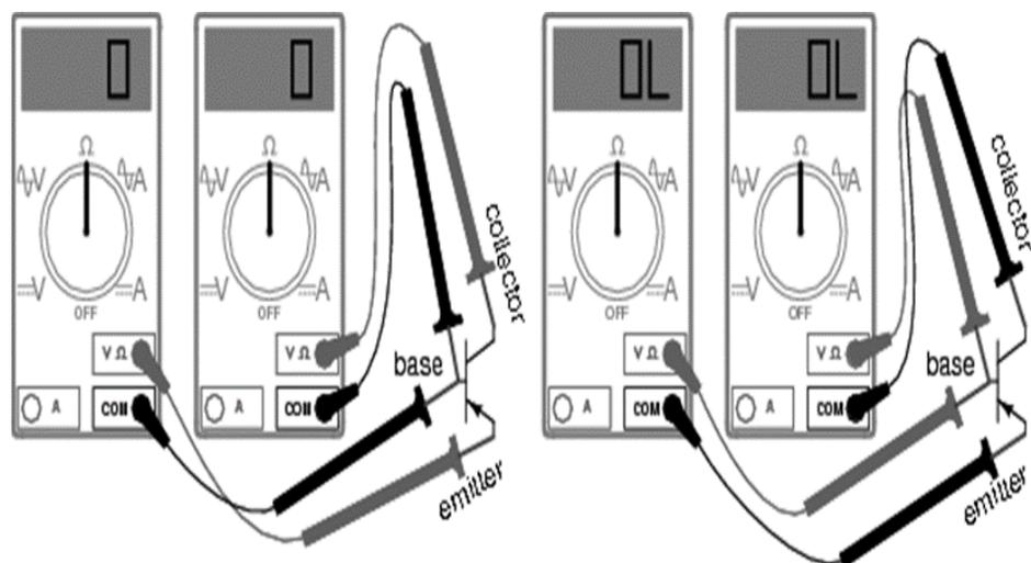
**Figure 14.3: Connection of transistor testing using DMM**
