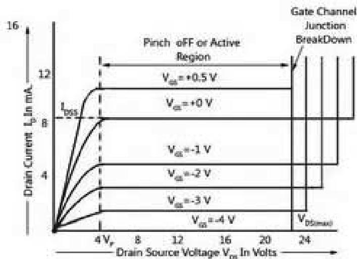
Figure 18.2: Drain characteristics
