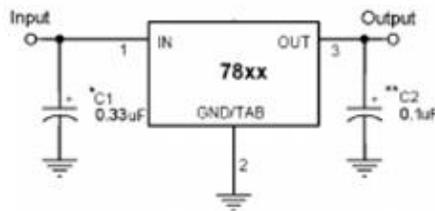
A common ground is required between the input and the output voltages. The input voltage must remain typically 2.0V above the output voltage even during the low point on the Input ripple voltage.
