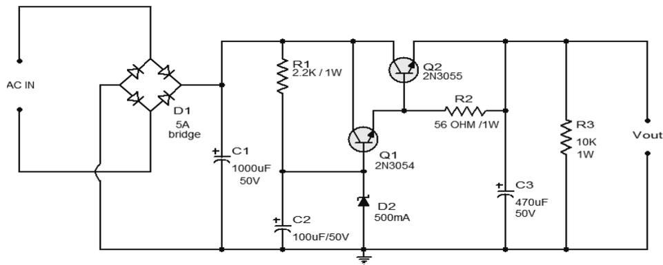
**Figure 22.1: Regulated power supply**
