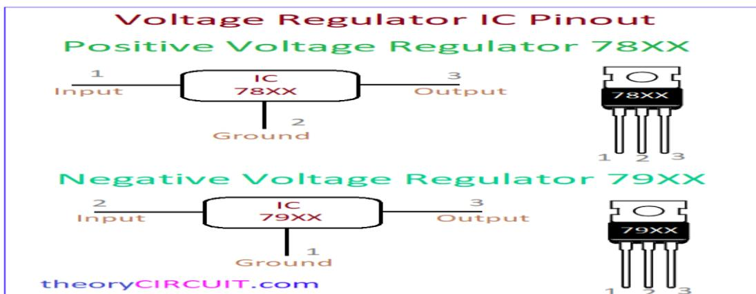
Figure 25.1: Pin diagram of IC78XX and 79XX
