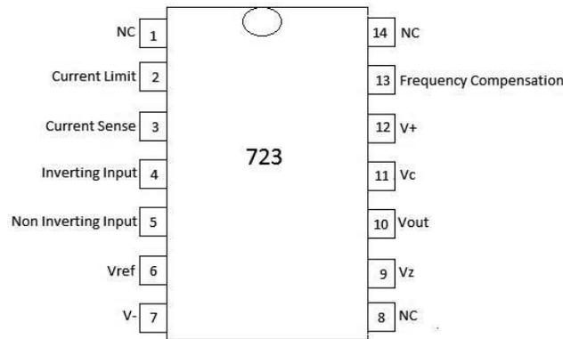
Figure 26.1: Pin diagram of IC LM723
