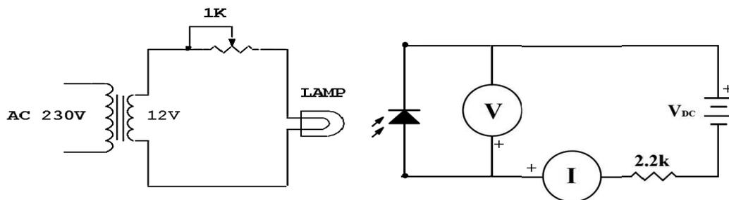
**Figure 5.4: Photodiode practical setup**
