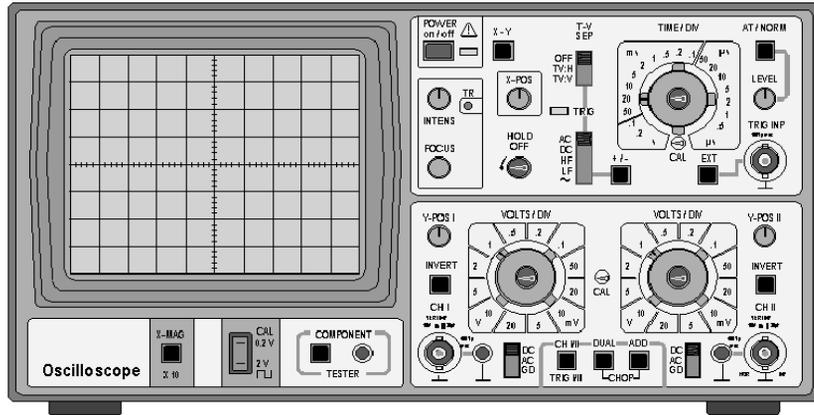
Figure 2.3: Front Panel of CRO
