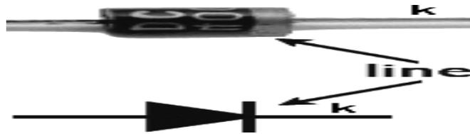
**Figure 3.1: Diode and its symbol**
