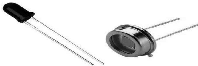
**Figure 5.2: Photo Diode**
