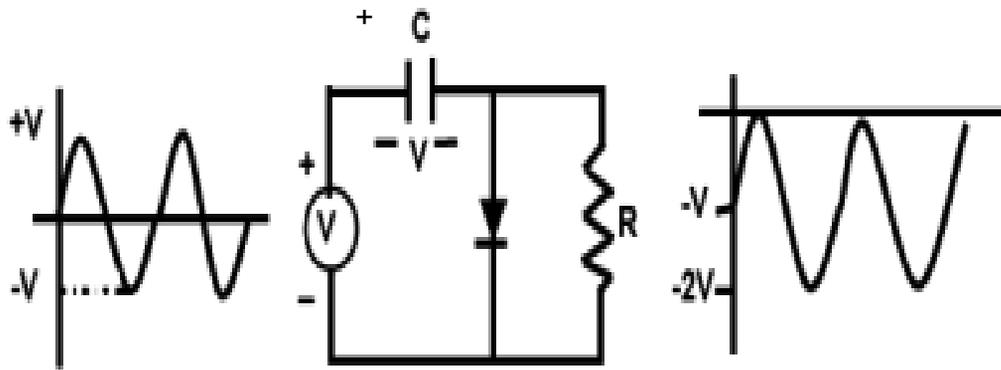
**Figure 13.2: Circuit diagram of Negative clamper.**
