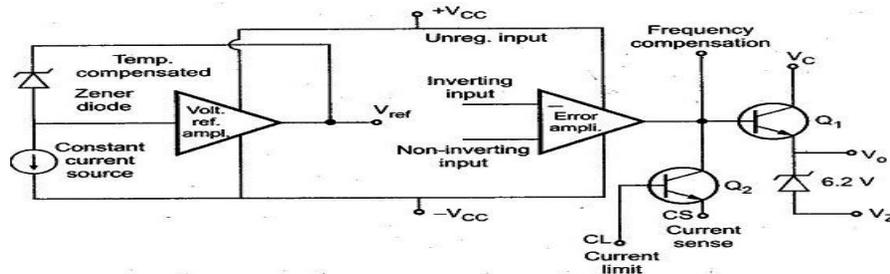
Figure 26.2: Block diagram of IC LM723
