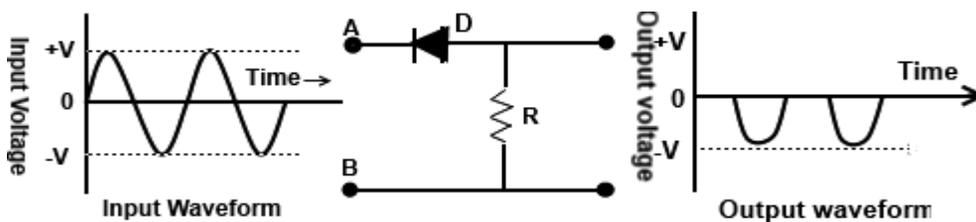
Figure 12.1: Circuit diagram of Positive Clipper.
