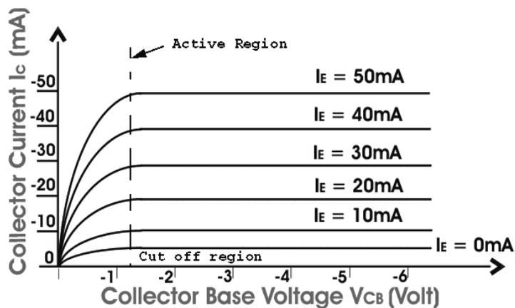
Figure 15.2: Output characteristics in CB
