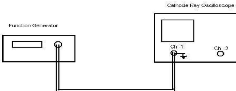
Figure 2.5: Connecting Function Generator to CRO
