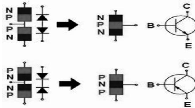
**Figure 14.1: Symbol and construction of NPN and PNP transistor**
