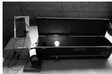
Fig. To determine characteristics of photoelectric cell
