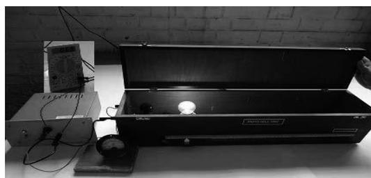
**Fig (1) To determine characteristics of photoelectric cell**
